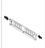
Figure 11. Installing the memory module
